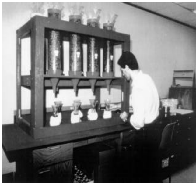
Figure 5.2. Leaching Columns (from Bradham and Caruccio, 1995)
